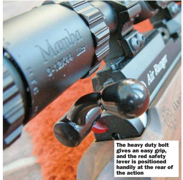
The heavy duty bolt gives an easy grip, and the red safety lever is positioned handily at the rear of the action
