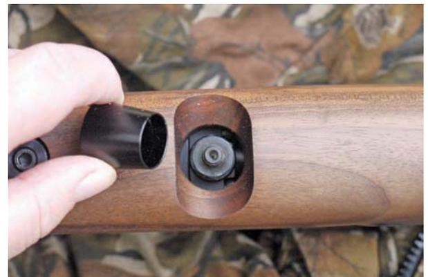
The air bottle is filled via a quick fill valve at the base of the action – note the push fit dust cover
